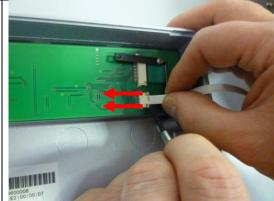
14 Pivot the black retaining clip back in position and tighten the screws. WARNING: the LCD flex cable is located very close to the mounting screw thread, make sure not to damage the flex cable when fixing the screws.
