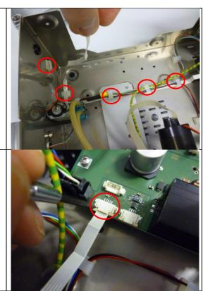
Take the new flex cable and insert it in the corresponding connector on the LCD circuit board. Slide the connector in as far as possible with the contacts facing upwards. Fix the cable by pushing the retaining clips on both sides in the direction indicated by the arrows as far as possible. Do this very gently.
